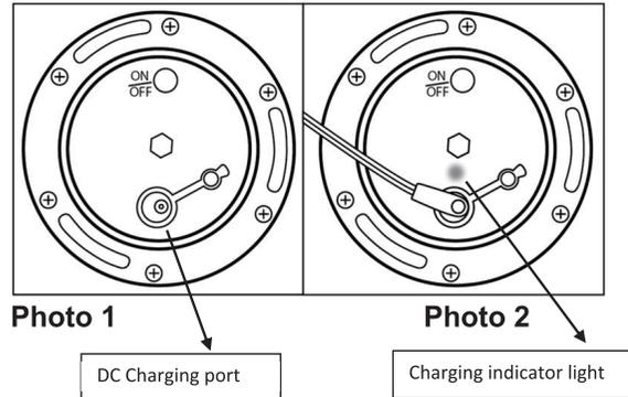
To turn on/off the product by pressing bottom ON/OFF switch or directly pressing ON/OFF button on remote control.
